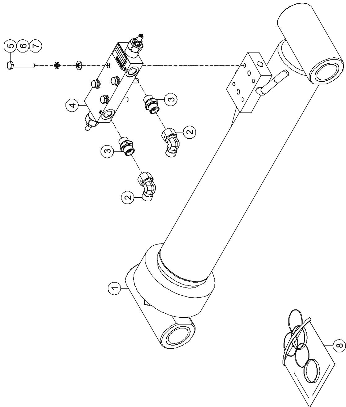
**5-5 JIB Leveling Cylinder Assembly (BT22RT)**
