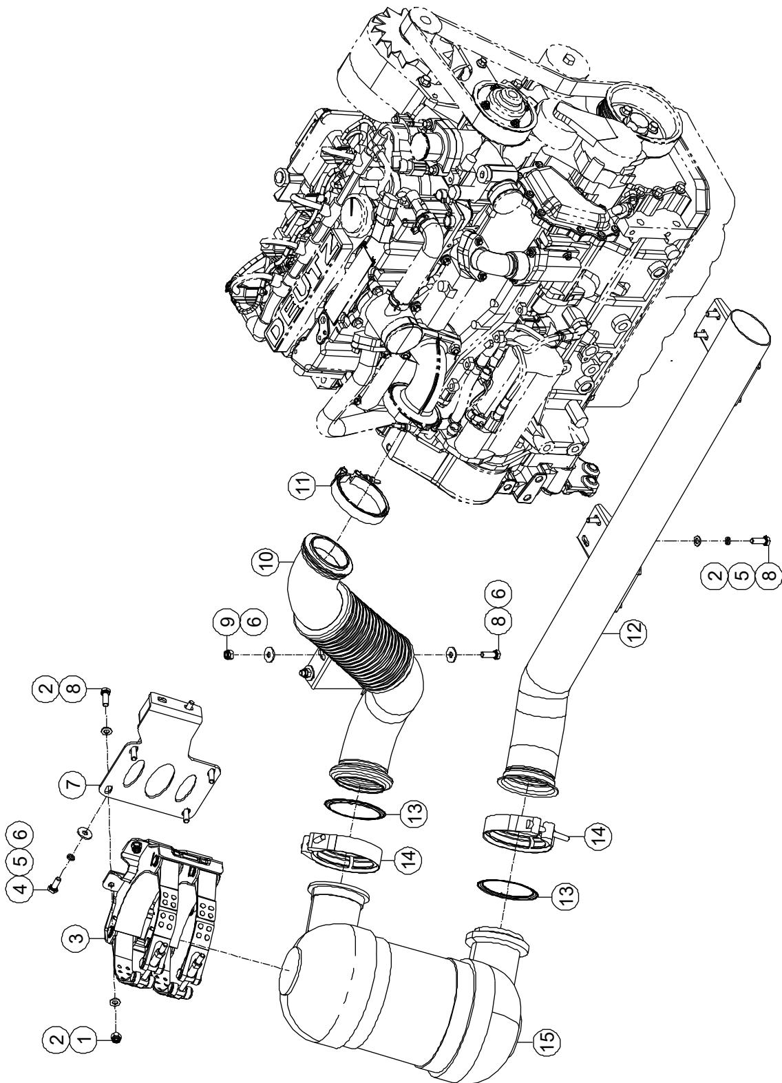
**1-24 Engine Exhaust System Installations (Stage IV)**
