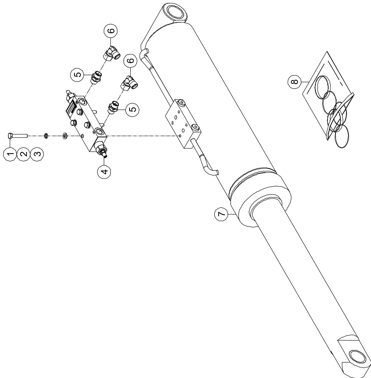
**5-6 JIB Leveling Cylinder Assembly (BT22BRT)**
