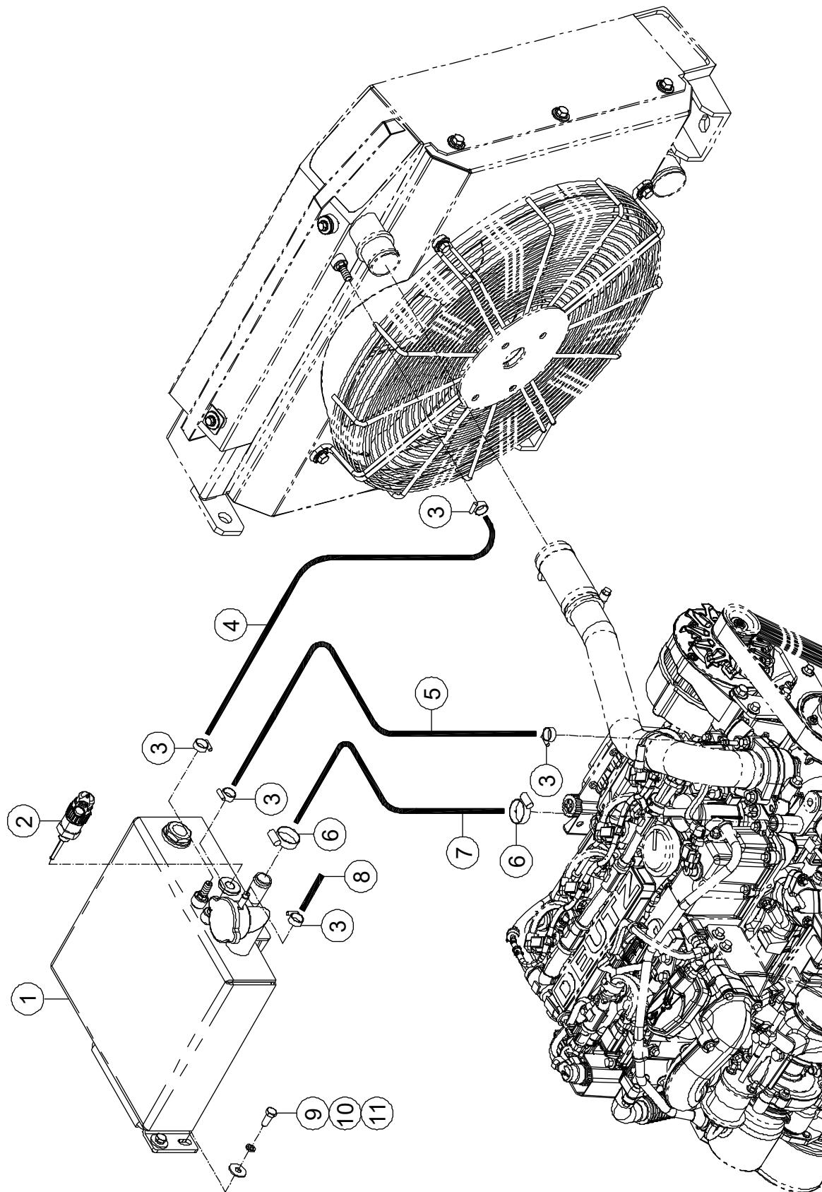
**1-18 Engine Cooling System Installations 2 (Stage V)**
